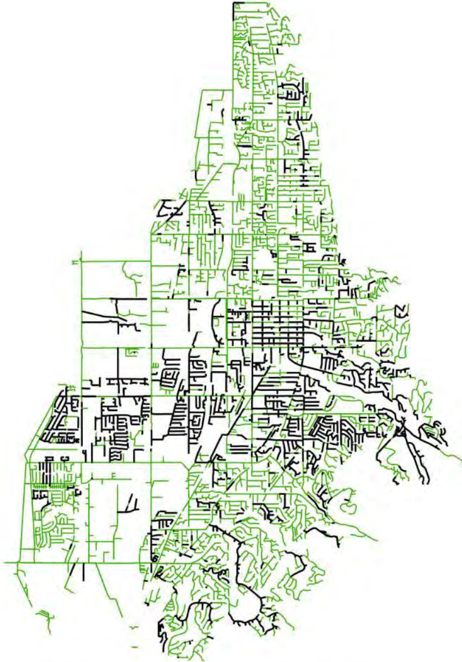
Pipe sections that were TV'ed between 2020 and 2022 are shown above in black.
